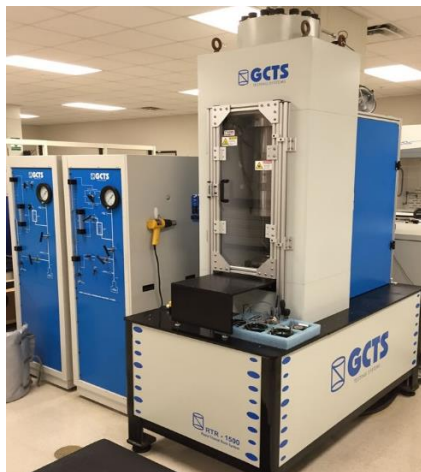
Figure 1: Triaxial pressure vessel for rock mechanics testing
