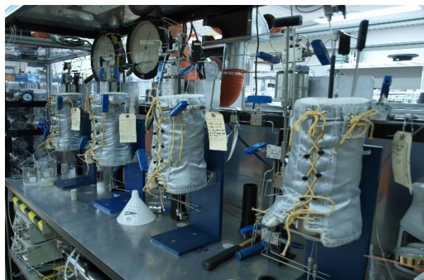
Figure 1: The steady state permeability apparatus used in this example had the capacity to measure permeability on four 1" \varnothing core plugs simultaneously.
